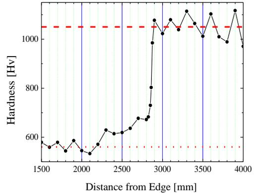
Fig. 7. Surface hardness profile in the vicinity of the boundary of treated and untreated area.
