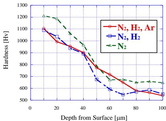
Fig. 6. Hardness gradient for several treatment gas.
