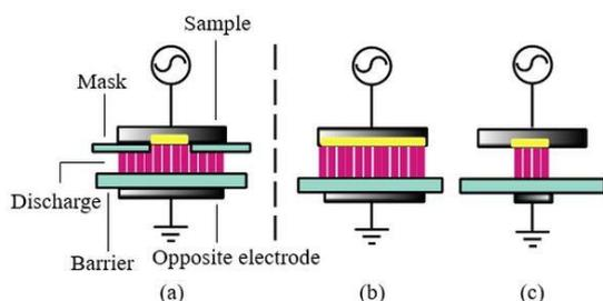
Fig. 1 Schematic of large area treatment and mask-free patterning by DBD. (a) Conventional patterning with masking. (b) Large area treatment. (c) Mask-free patterning.
