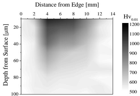
Fig. 5. Hardness profile of sample cross-section.
