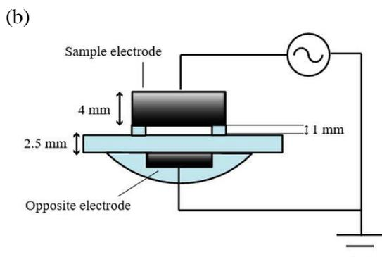
Fig. 2. Schematic of experimental setup. (a) Treatment furnace. (b) Electrode system.
